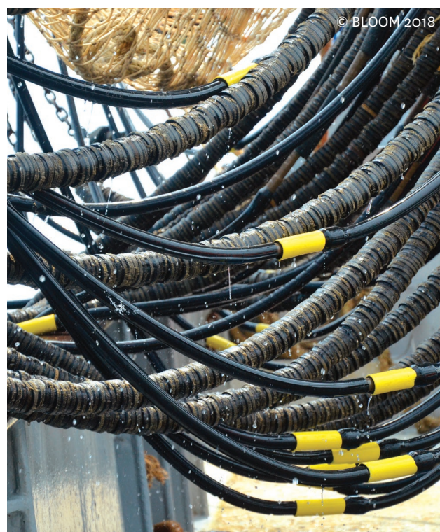
Focus on cables on an electric 'pulse' trawl.
